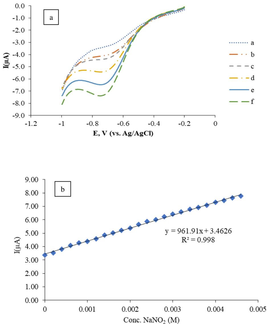
**Fig. 5.** (a) Typical LSV curves of different concentrations of nitrite on GCE/PPy/Hb in 0.1 M acetate buffer (pH 4.5), Concentration of nitrite (a-f): 0.000, 0.0006, 0.001, 0.002, 0.003, and 0.004 M. Scan rate 0.100 V/s. (b) Calibration curve for different concentrations of nitrite at the optimum condition.
